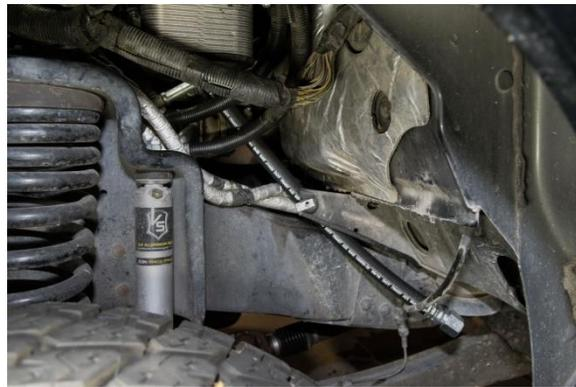
5. Connect the 90° fitting on the top side to the "Oil Out" fitting on the OEM Engine Oil Cooler Plate.
