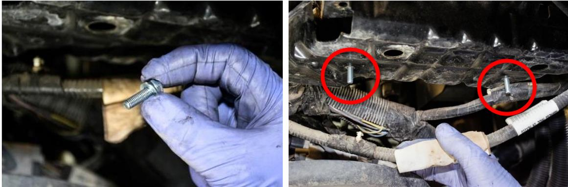
13. Slide the oil cooler bracket into place, making sure to locate the rubber isolator with the appropriate holes in the oil cooler bracket.
