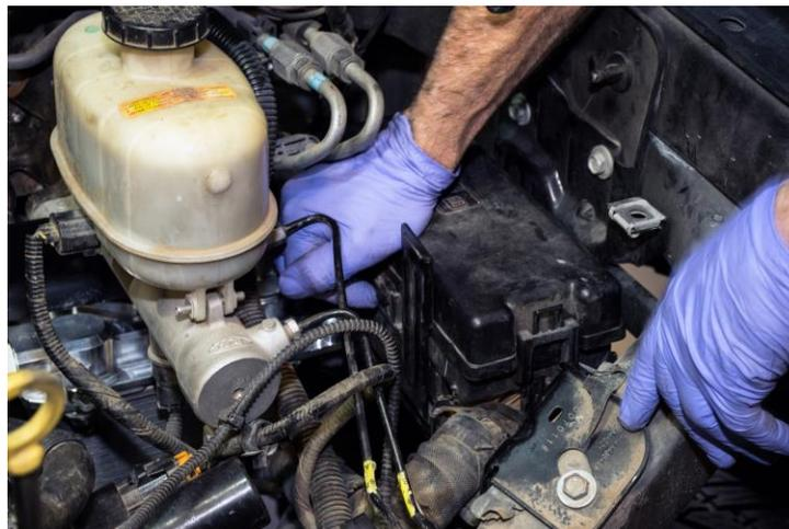
18. Use the two provided zip tie connectors to re-secure the wiring harness to the newly installed plate.
