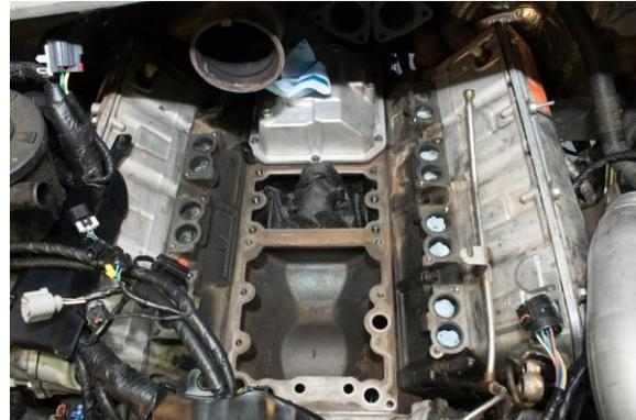
3. Install the provided seals into the bottom of the oil transfer plate; be sure to fully seat the seals into the transfer plate.
