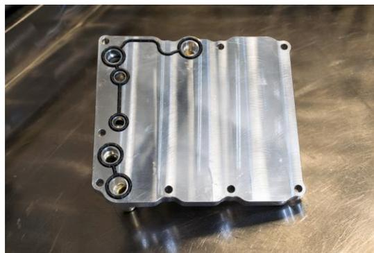
4. Remove your existing oil temperature sensor and oil pressure sender from the OE oil cooler cover and install those into their respective holes in the oil transfer block.
