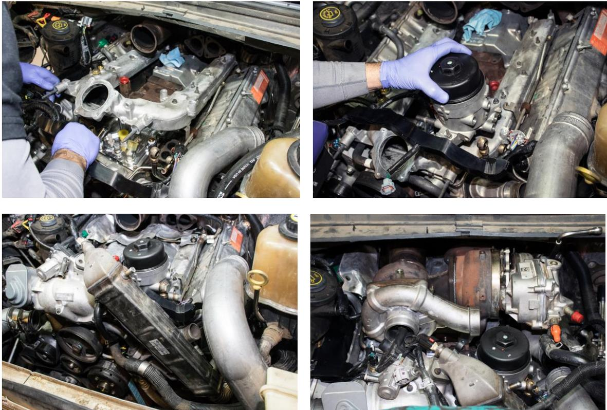
**Note:** Leave the u shaped portion of the turbos on the driver's side of the engine off until the oil cooler/oil cooler plate is installed and hoses are hooked up, this will come in the next section of the manual.
