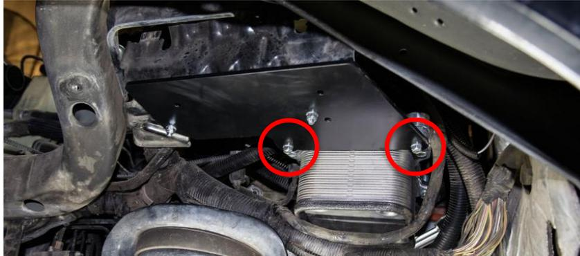
16. Now tighten the remaining lock nut on rubber isolator.
