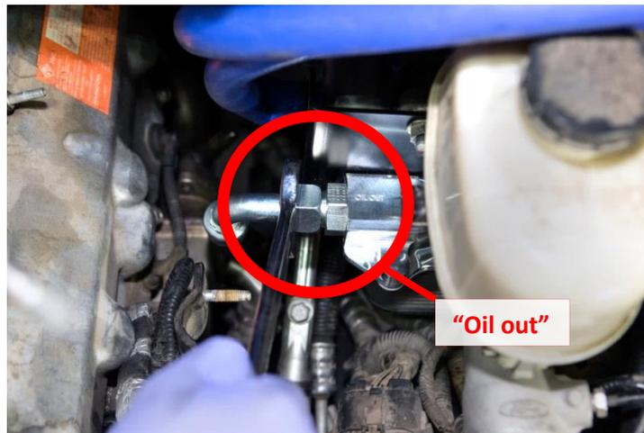
6. Connect the straight fitting on the underside to the 90 degree fitting, or the "Oil In" on the Oil Filter Housing.
