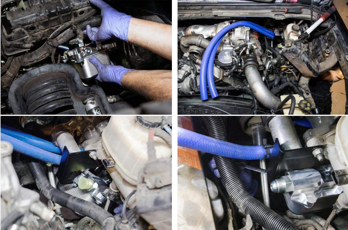
11. Slide the oil cooler into place before installing the bracket.
