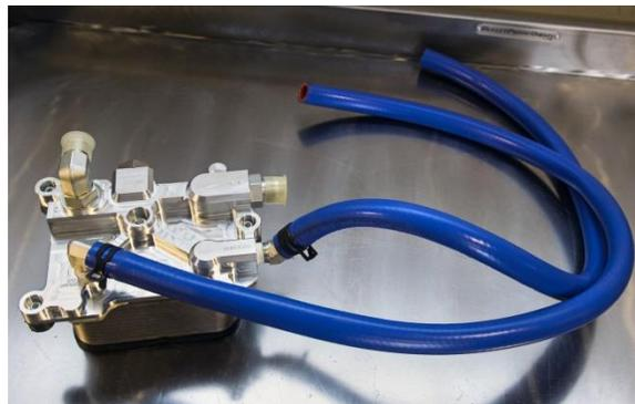
10. With coolant hoses installed, slide the oil cooler / hose assembly through the void on the inner fender on the driver's side. Guide coolant hoses over turbo while sliding oil cooler into place.
