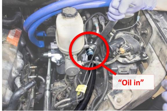
4. Install the 90°x0° 38.5" hose by guiding the straight end of the hose down towards the oil filter housing, guide the hose to the left of the steering rod as shown.
