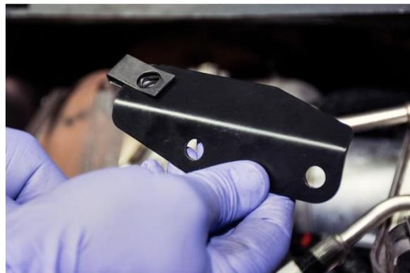
2. Index the bracket on to the fuel cooler mounting studs. Install the two retaining nuts.
