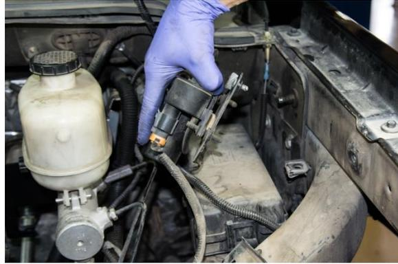
6. Unclip all four retainers to release the fuse box from its bracket.
