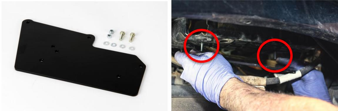
14. Once the bracket is in place, install the two retaining nuts on the bracket.
