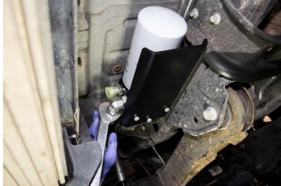
7. Next, connect the 90°x0°, 88" hose by guiding the straight end of the hose up into the engine compartment through the wheel well as shown. Guide the 90° fitting alongside the other oil line to the oil filter housing. Tighten the 90 degree end of the hose to the straight fitting, or the "Oil Out" on the Oil Filter Housing.
