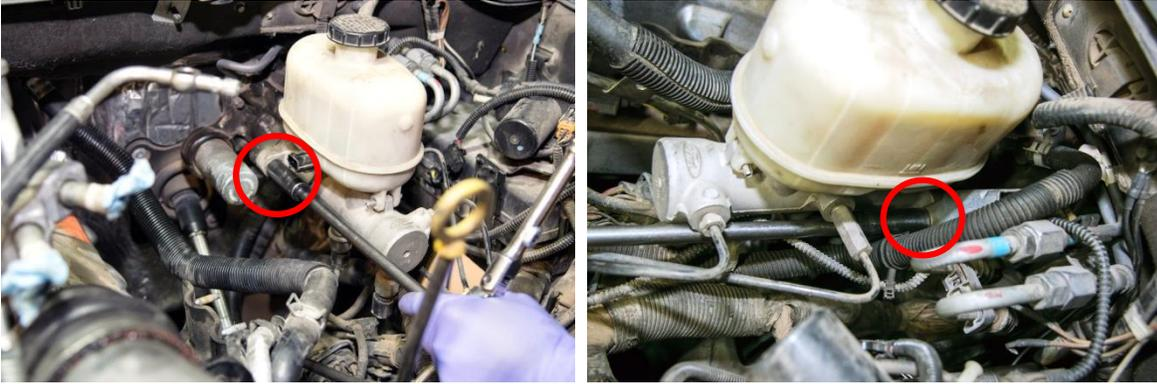
4. Using the supplied bracket, install over the brake master cylinder studs and replace the two retaining nuts.
