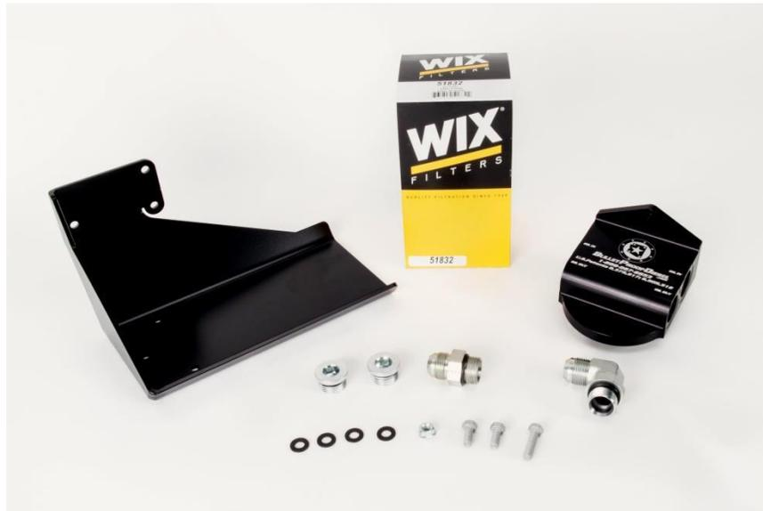
1. Install the fittings and the plugs into the oil filter adapter. We recommend using a lubricant on the O-rings to help seat the fittings. Leave the 90 degree fitting clocked as shown; do not tighten the jam nut all the way, this will allow you to re-position the fitting during the hose installation.
