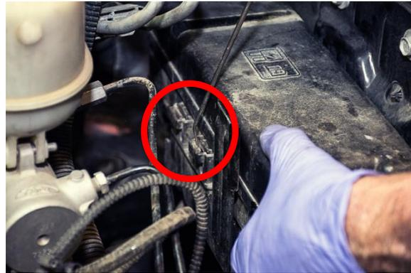
7. Accessing from the inner fender well, unclip wiring harness from the fuse box bracket.
