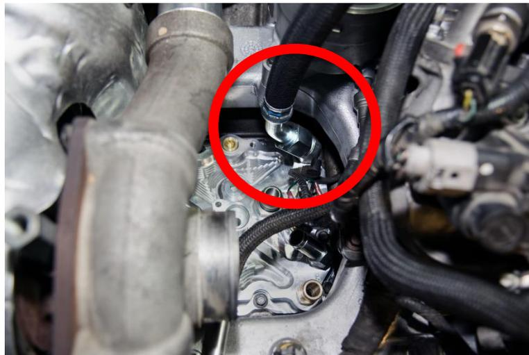
3. Route the hose around the fuel filter cap and under the CAC (Charge Air Cooler) pipe, continue the routing under the degas bottle hose elbow and tubes as shown. Tighten the straight end to the "Oil In" fitting on the OEM Engine Oil Cooler Plate as shown.
