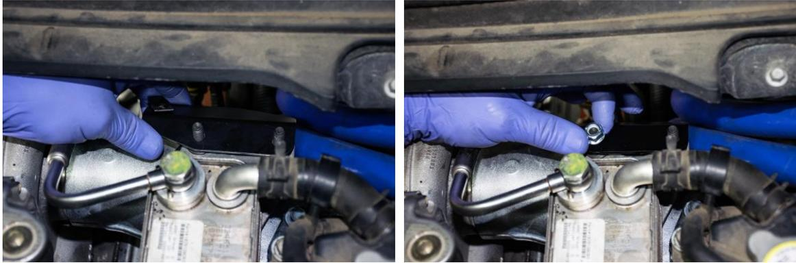
3. Install the rubber dipped clamps on to the coolant hoses, then slide the bolt through the rubber dipped clamps and tighten to the bracket.
