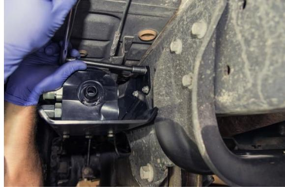
5. Install the provided filter onto the oil filter adapter.
