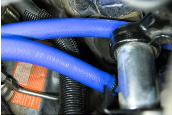
**TIP: Check lines by the heater hose: the front hose (shorter) may go over or under the heater hose to prevent kinking. Use whichever method works best on your vehicle.**
